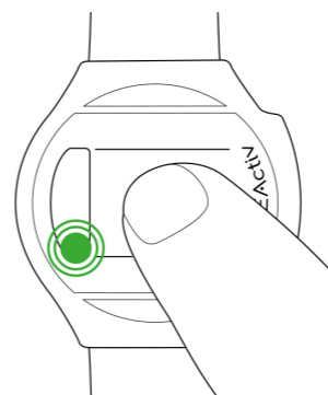
Long Flash (in button start mode) = recording started Short Flash (when unconfigured) = battery good for storage
